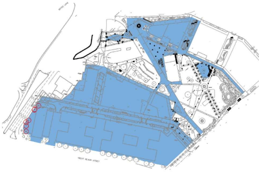
Proposed Impermeable Area 3.4ha Restricted run off rate 154l/s
